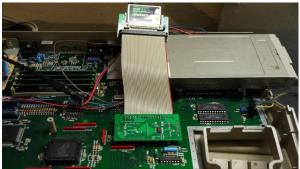
Don't forget to power up your device (internal or external). You will have to find a way to do that since there is only one plug for the drive (add a plug by soldering it to the motherboard, external powering, etc.)
